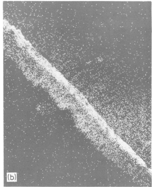
Figure 7 Another part of the specimen shown in Fig. 5. (a) SEI, (b) Ag X-ray image, (c) SEI of the same area after recording (b).
